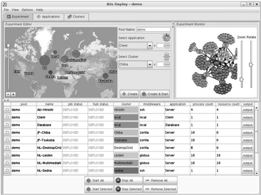
Fig. 8.4 The IbisDeploy GUI that enables runtime loading of applications and resources ( top middle ) and keeping track of running processes ( bottom half ). Top left shows a world map of the locations of available resources; top right shows the SmartSockets network of hubs. See also http://www.cs.vu.nl/ibis/demos.html
